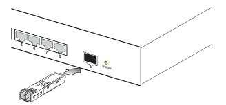
Figure 3-5 Inserting an SFP Transceiver into a Slot
